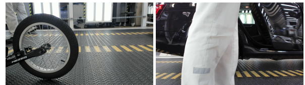
Fig. 4. Examples of problematic objects in the scene: a scooter wheel is not the object of interest, and a staff standing in front of the car completely occluding the wheel.
